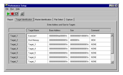
In this table you can specify up to ten different target devices including their address ranges and the types of PCI commands that are considered in the measurements.
