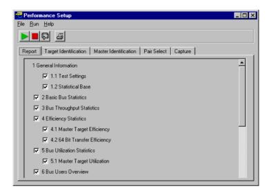
After the test has finished, the software provides a textual report of the results in the Performance Report window. With the items found on this tab of the Performance Setup window you can specify the particular results and statistics that are included in the report.
