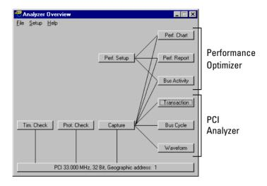
This Analyzer Overview window shows the individual components of the PCI Analyzer and the PCI Performance Optimizer and how they interact. Clicking the buttons brings up the respective windows.
